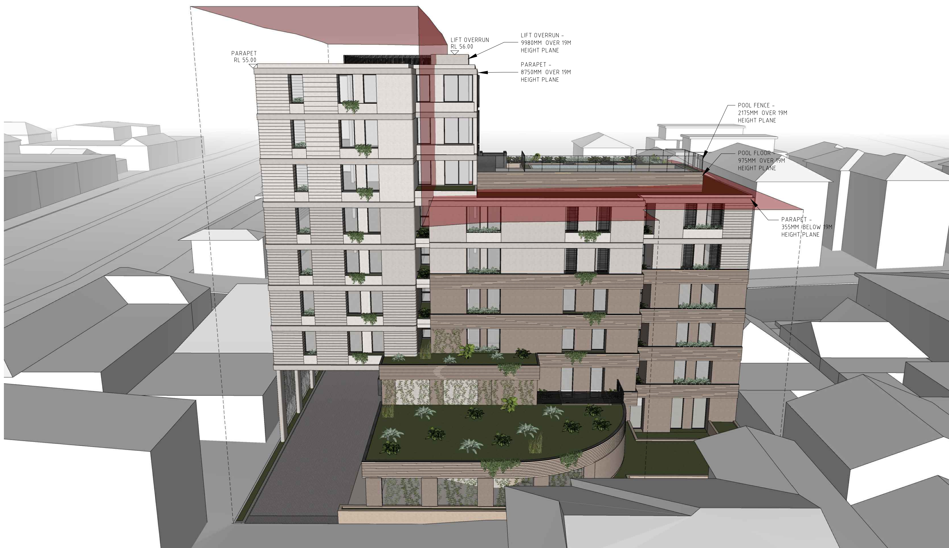
2 COUNCIL BUILDING HEIGHT CONTROL PLANE AERIAL VIEW FROM SOUTH w/ RLEP 31/19M COUNCIL HEIGHT OF BUILDING CONTROL PLANE
